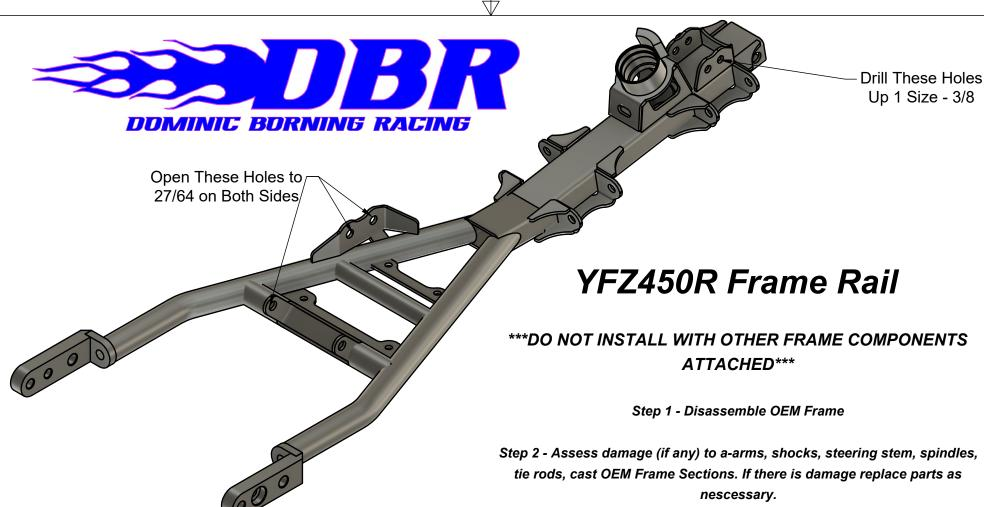
Step 3 - With all cast aluminum components loose. Start bolting them together being sure to leave them loose until they are installed. Use OEM Torque Specs.
